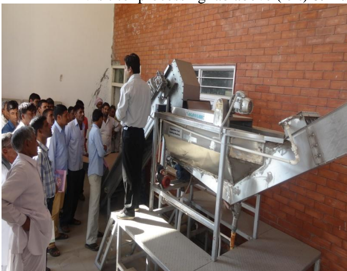
Conveyer belt to receive fruits after automatic grading (left) and cutting machine (right)
