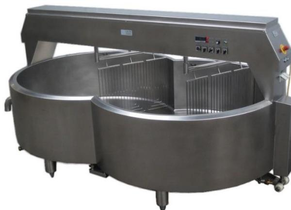
c) Horizontal enclosed cheese making machine with combined stirring and cutting tools and hoisted drain system:
