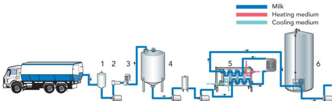
**Fig. Milk reception and pasteurization unit – Tetrapak Handbook:** a) Air eliminator, b) Filter, c) Milk meter, d) Intermediate storage tank, e) Thermization/pasteurization and cooling, f) Silo tank
