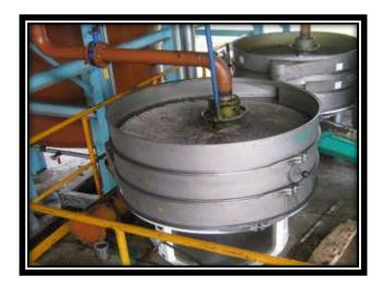
**3.5 GRAVITY SEPARATOR:** Gravity separator machine may be used to separate any type of dry bulk particles that are similar in size and shape but differs in weight. Gravity separator are suitable for processing of the seeds of corn, Wheat, rice, soybean, sorghum, various vegetables and other agricultural and sideline products.
