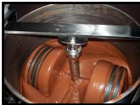
Figure 17. A typical conching machine
