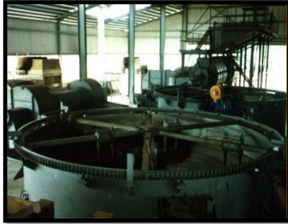
Figure 11. Mechanical drying of cocoa beans
