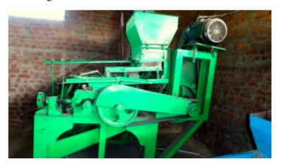
Fig. 8 Roller machine for making thin flaked rice
