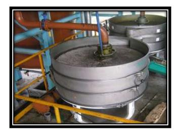
**3.6 GRAVITY SEPARATOR:** Gravity separator machine may be used to separate any type of dry bulk particles that are similar in size and shape but differs in weight. Gravity separator are
