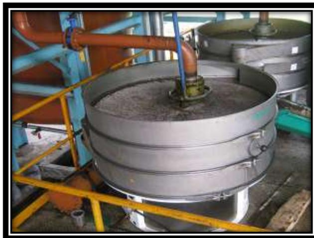
**3.6 GRAVITY SEPARATOR :** Gravity separator machine may be used to separate any type of dry bulk particles that are similar in size and shape but differs in weight. Gravity separator are suitable for processing of the seeds of corn, Wheat, rice, soybean, sorghum, various vegetables and other agricultural and sideline products.
