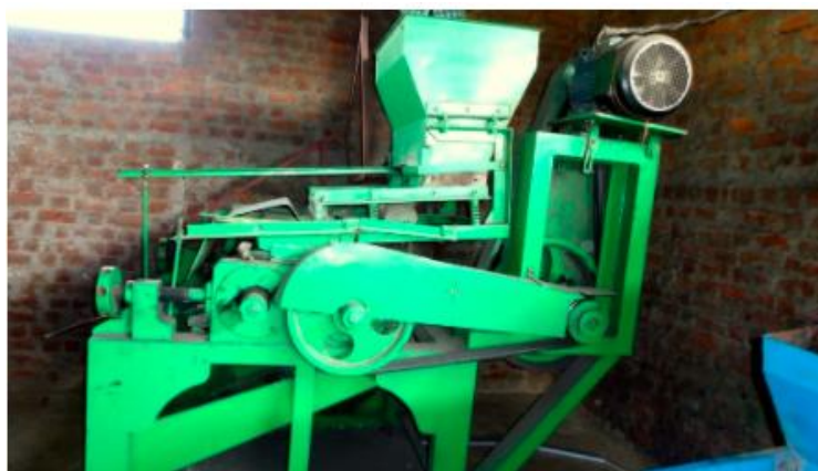
Fig. 7 Roller machine for making thin flaked rice
