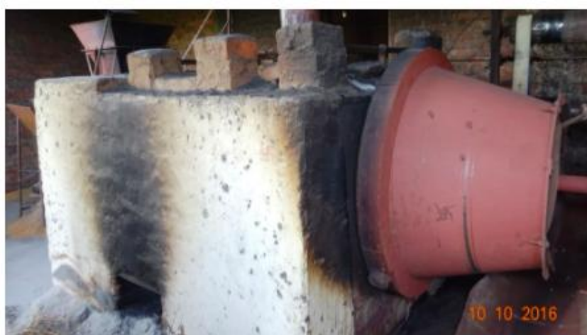
Fig. 5 Roaster machine for flaking process
