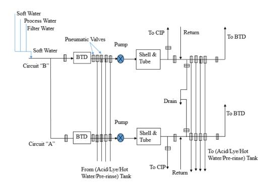
Fig: A two station CIP Circuit(model)
