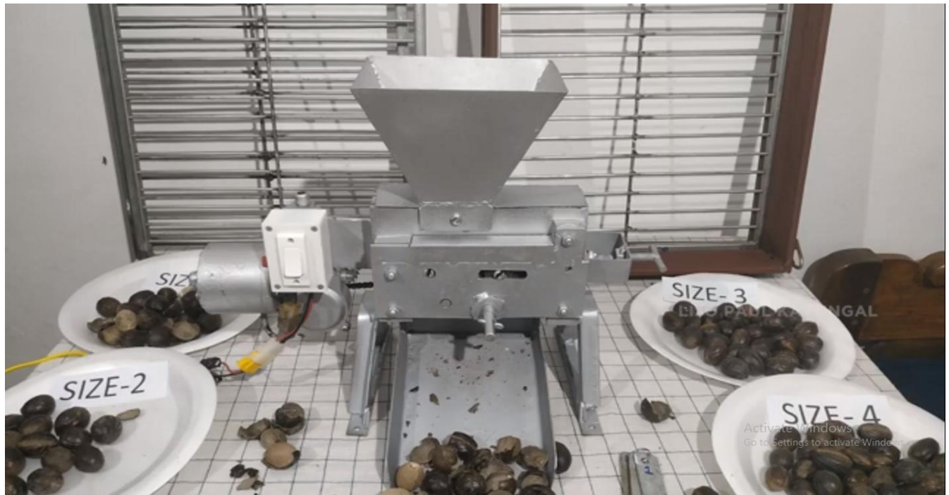
Figure 2: Nutmeg cracker and sorting meshes
