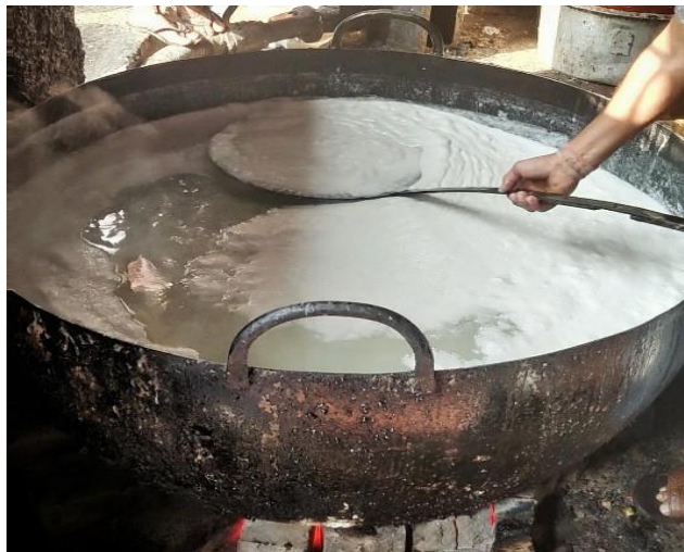
Fig 10: Removal of scum
