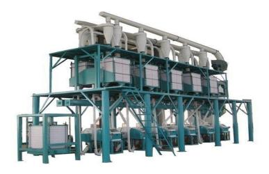
of milling it is necessary to collect the bran that has been sieved off during the early stages of milling and add them back to the final product. To obtain brown flour a proportion only of the extracted material is added back.
