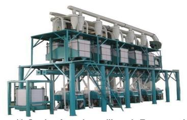
counter-rotating rollers with fluted surfaces, these mills work. To separate the bran from the starchy endosperm, the resulting crushed grain is sieved between each pair of rollers. It is a super-fine white flour that is the finished result. To produce wholemeal flour from this type of milling it is necessary to collect the bran that has been sieved off during the early stages of
