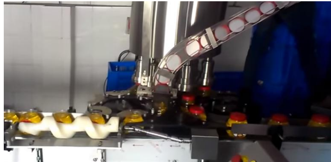
Lid placing and sealing
