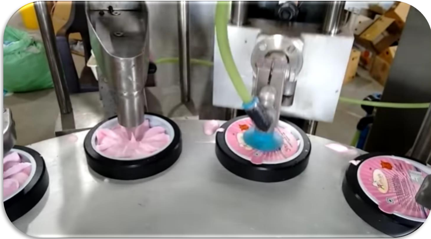
Ice cream cup filling and packaging line Source: Kunal International, Bengaluru
