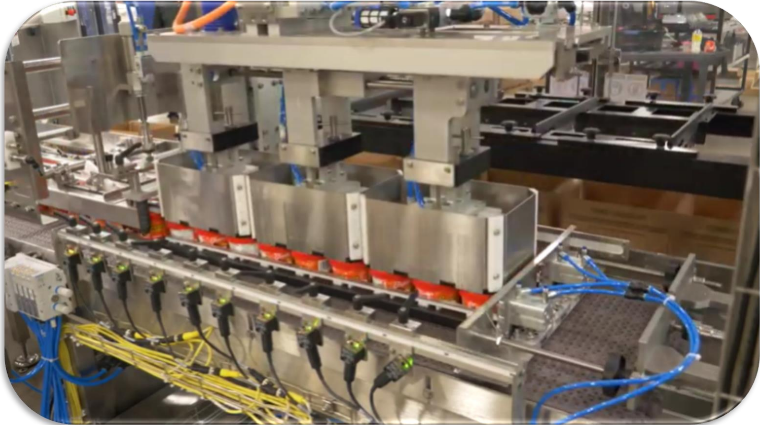
Ice cream packaging line (cups are putting in a carton) Source: Delkor Systems Inc.
