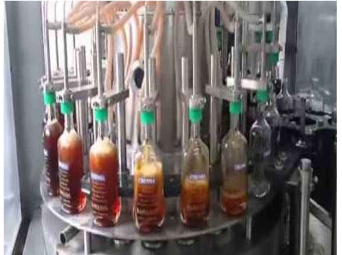
Automatic whisky bottle filling machine
