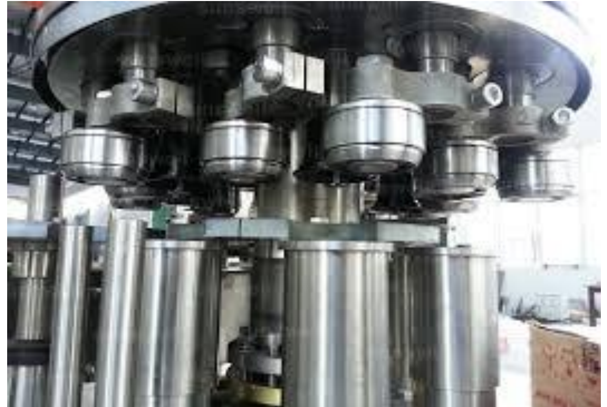
Can filling and seaming equipment
