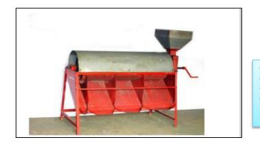
Feed Hopper Capacity – 200 Kg per Hour Efficiency - 88%
