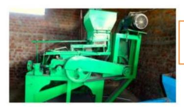
Roller machine for making thin flaked rice
