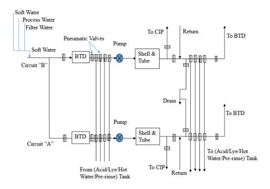
A two station CIP Circuit (model)
