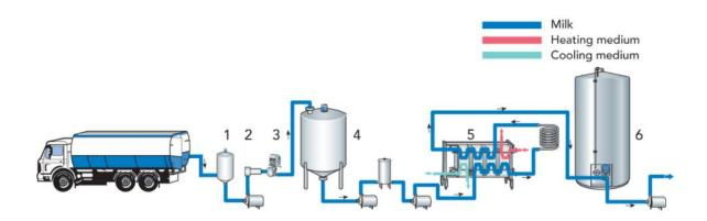
**Fig. Milk reception and pasteurization unit – Tetrapak Handbook:** a) Air eliminator, b) Filter, c) Milk meter, d) Intermediate storage tank, e) Thermization/pasteurization and cooling, f) Silo tank
