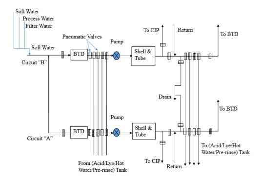
Fig: A two station CIP Circuit (model)
