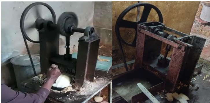
(a) Simple cutter (b) Pricking (Gudai) Machine
