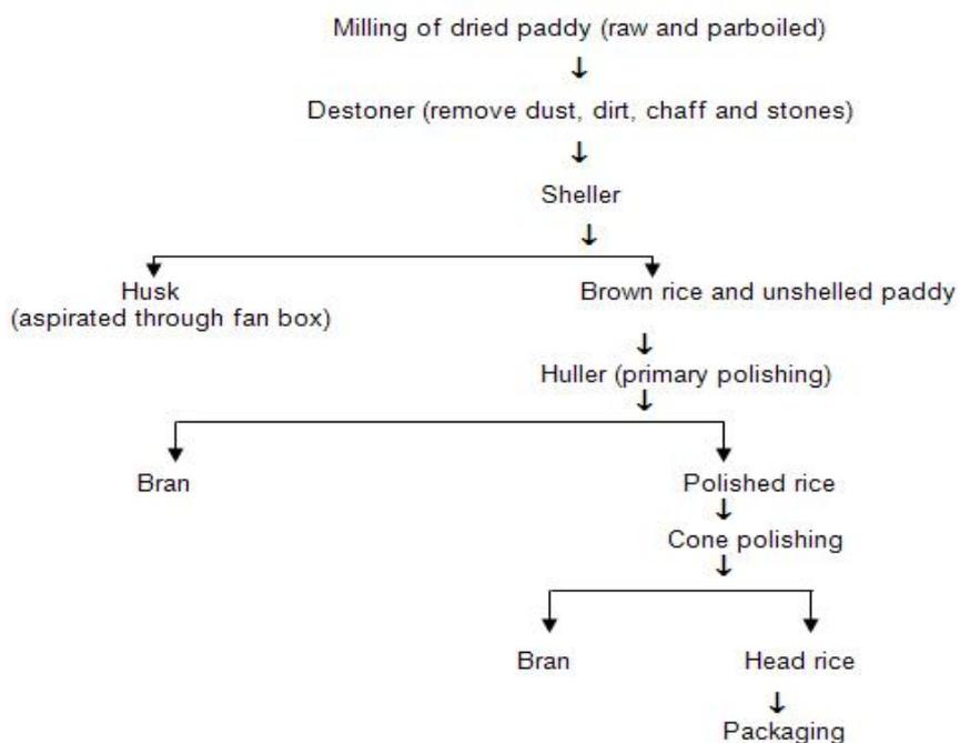
**Fig. 3 Process flow diagram of paddy milling**
