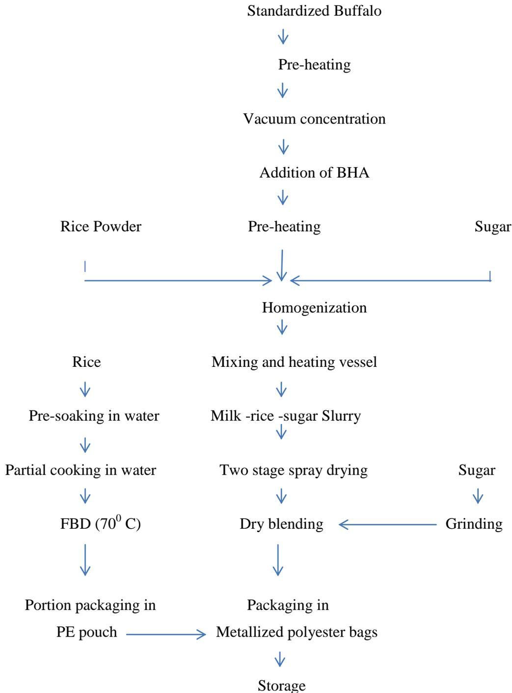
**Fig. 10 Flow chart for the manufacture of instant *kheer* mix.**
