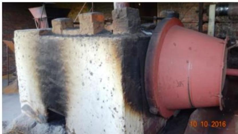
**Fig. 6 Roaster machine for flaking process**
