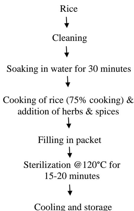
**Fig. 12 Process flow diagram of RTE rice processing**
