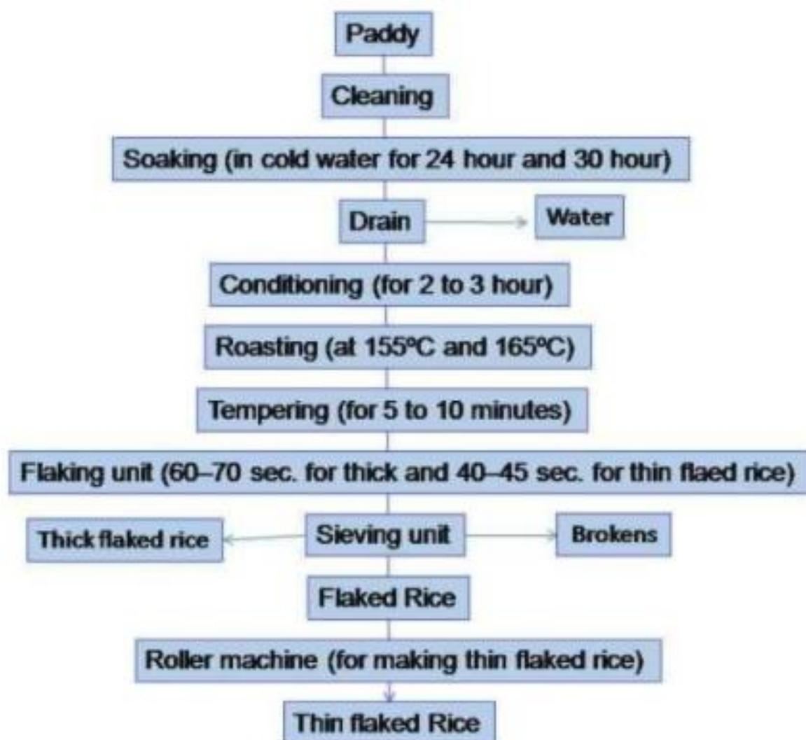
Fig. 5 Process flow chart for preparation of flaked rice
