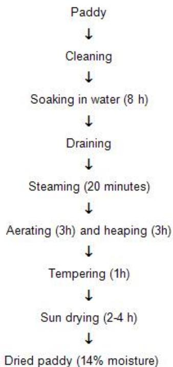
**Fig 2 Process flow diagram of parboiling**
