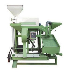
single-phase electric motor. This mill can readily dehusk strong pulses like tur, Bengal gram, field bean, and others.
