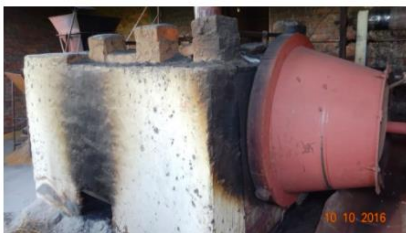
Fig. 5 Roaster machine for flaking process
