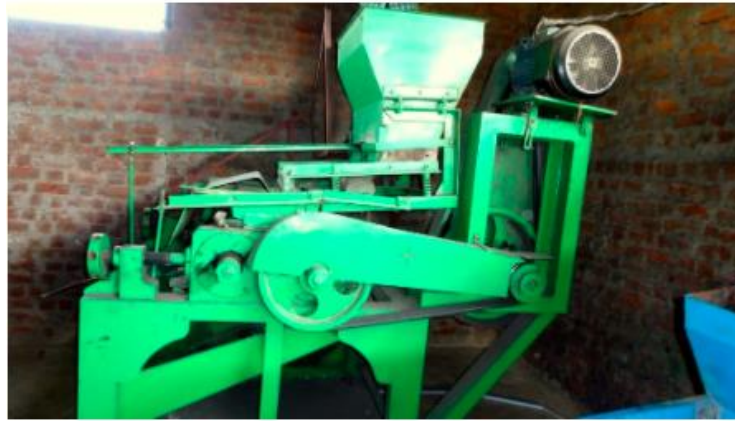
Fig. 7 Roller machine for making thin flaked rice
