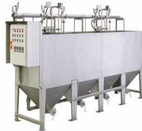
Soaking and washing machines
