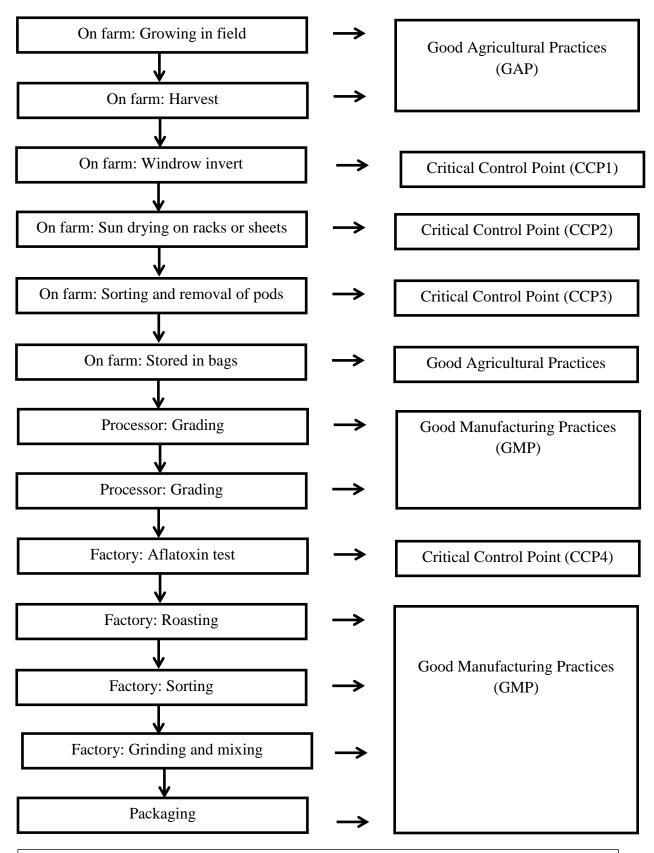
Figure 4: The hazard analysis and critical control point analysis for the peanut butter plant(FAO, n.d.)
