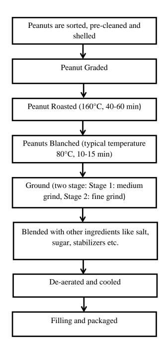
Figure 2: Flowchart for the peanut butter preparation process (Source: GAIC, 2017)
