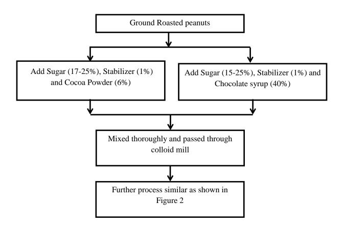
Figure 5: Variation in process flow for preparation of choco-peanut spread (Galvez et al. 2006).
