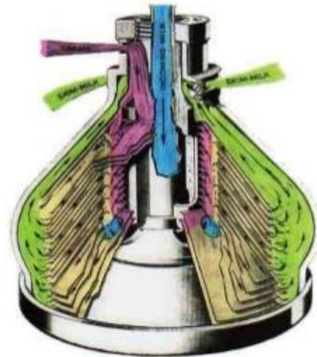
Blue - incoming whole milk Pink - separated cream Yellow - skim milk moving down cones Green - skim milk moving up & over cones
