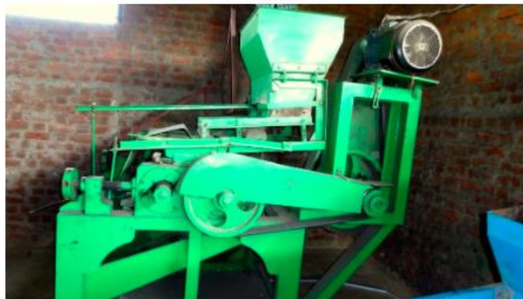
Fig. 7 Roller machine for making thin flaked rice
