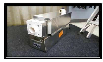
■ RETORT : Retort is used for sterilization of can so that microbial load can be reduced.
