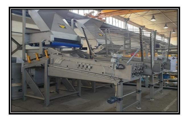
■ **DE SILKING MACHINE**: This machine is used for the removal for silk from the corn.
