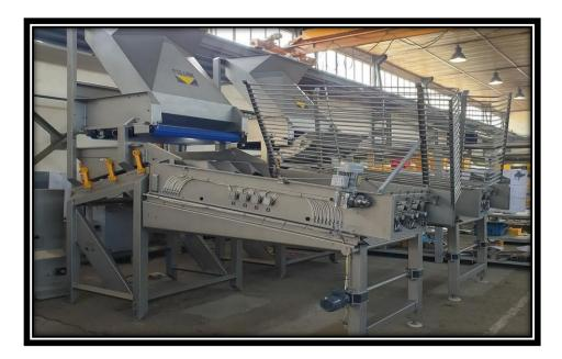
**3.2 DE SILKING MACHINE :** This machine is used for the removal for silk from the corn.
