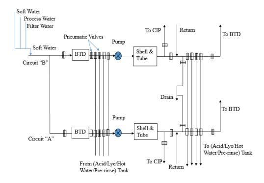
Fig: A two station CIP Circuit(model)
