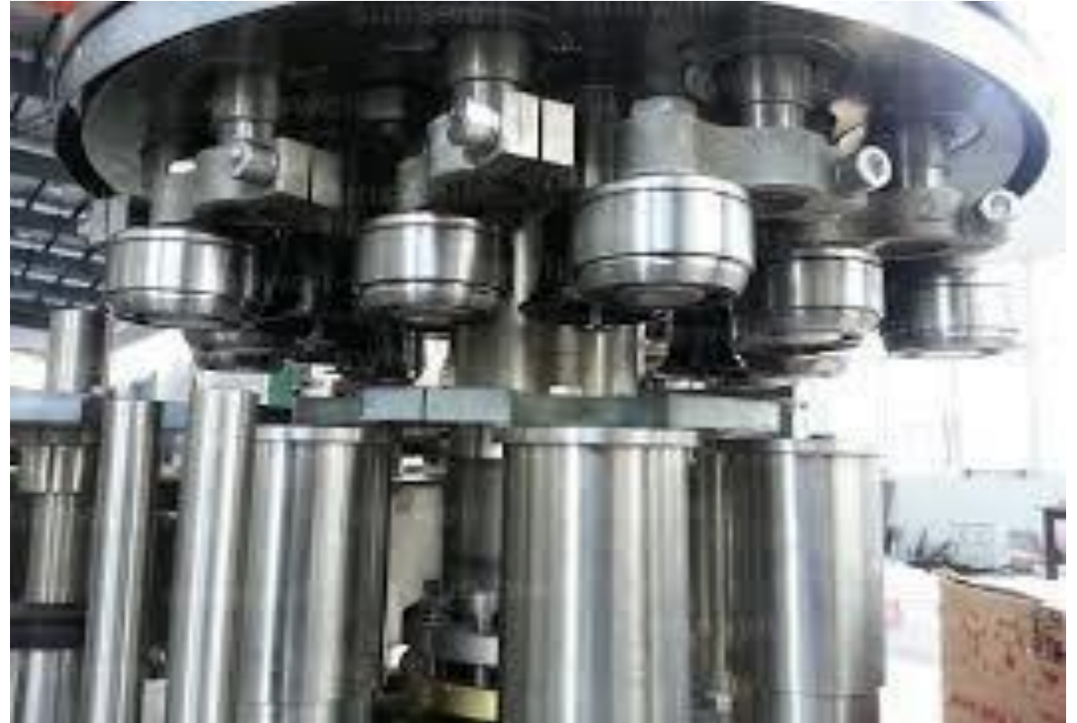
Can filling and seaming equipment
