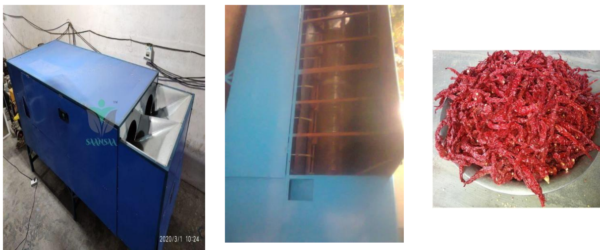
Fig. 2.1. Chilli stem cutting machine, its working components and chillies without stem
