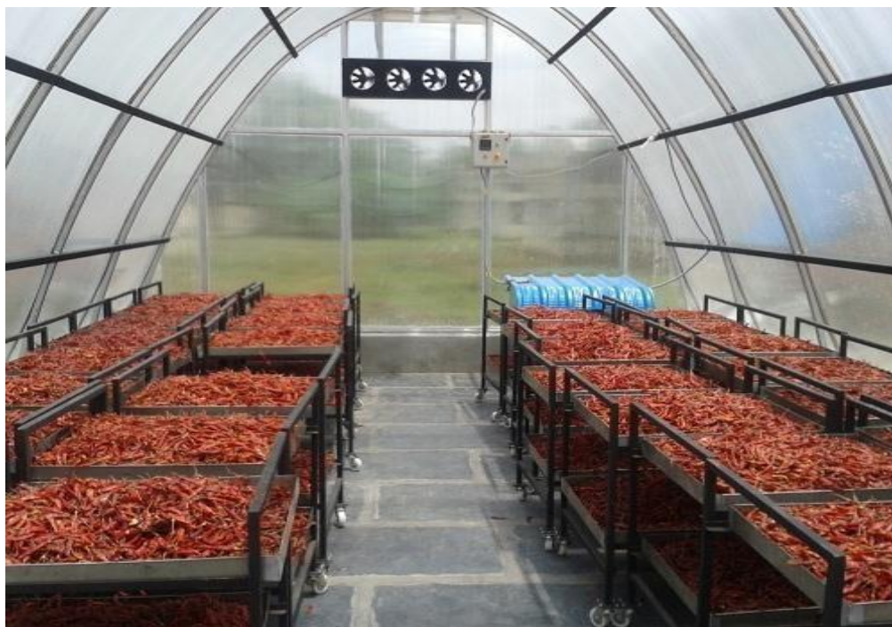
Fig. 1.7. Solar tunnel drying of chillies
