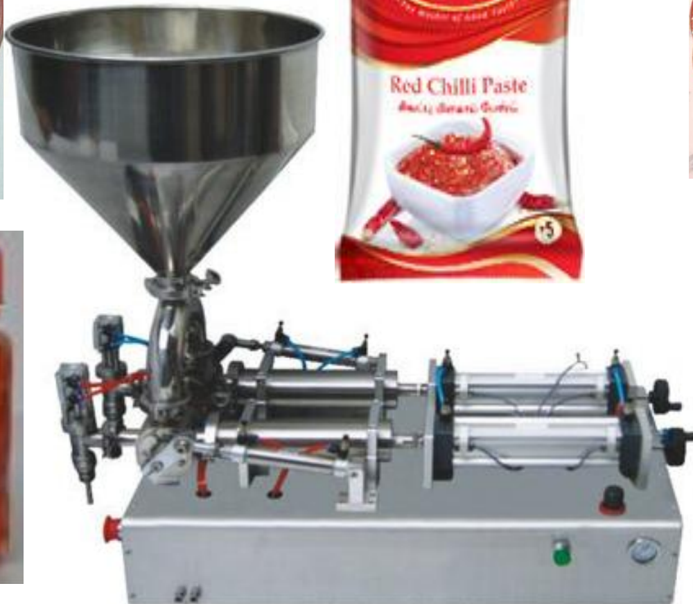
Double head paste filling machine
