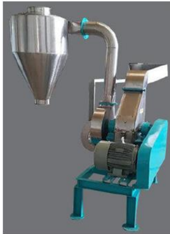
Hammer mill with centrifugal blower and cyclone separator
