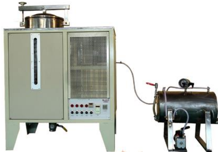
Solvent distillation unit
