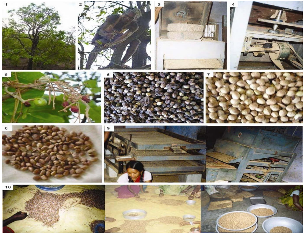
Fig: (1) Chironji tree; (2) Manual harvesting; (3) Traditional sheller for Chironji kernel shelling; (4) Driving mechanism of sheller (under runner) at cottage level; (5) Chironji leaves with immature nuts; (6) Harvested stored nuts; (7) Cleaned nuts; (8) Chironji kernels; (9) Grader for grading at cottage level; (10) Manual separation of kernels from hull and brokens
