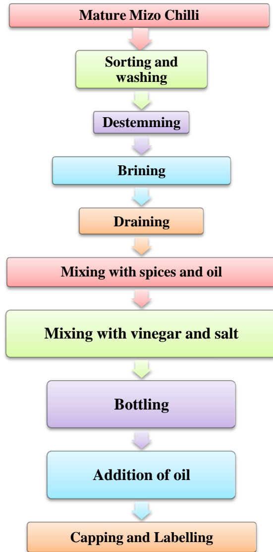
Fig. 2.8 Process flow chart for Mizo Chilli oil pickle
