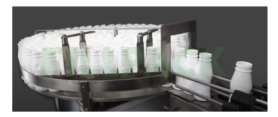
• PP bottles placed in a turn table and allowed to move on the conveyor belt (Picture source: FILLPACK TECHNOLOGY.)
