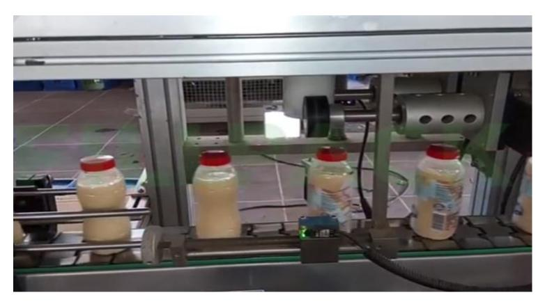
• PP bottles sleeving on the conveyor belt (Picture source: FILLPACK TECHNOLOGY.)
