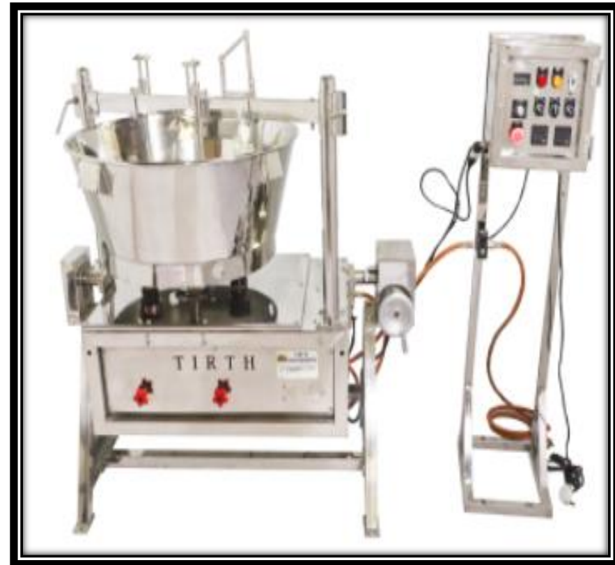
Multipurpose VAT (Rotating type / rotary scrapper)
