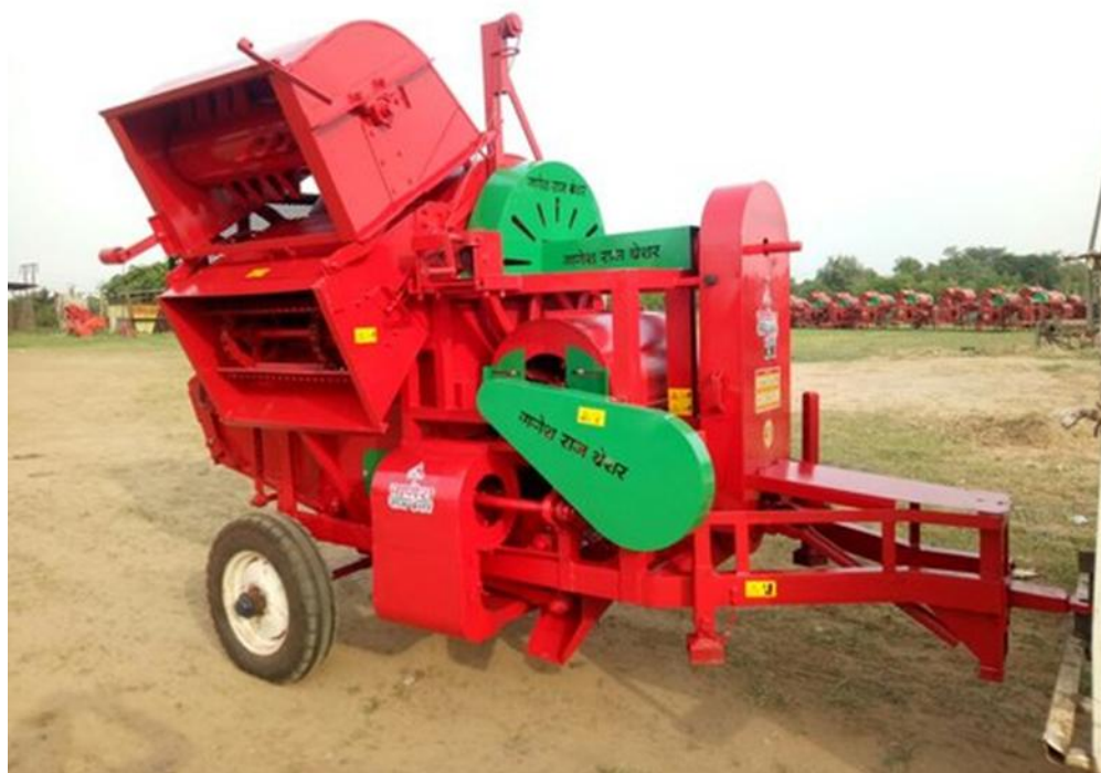
Figure 4: Groundnut pod thresher (1000-1500 kg / hr)
