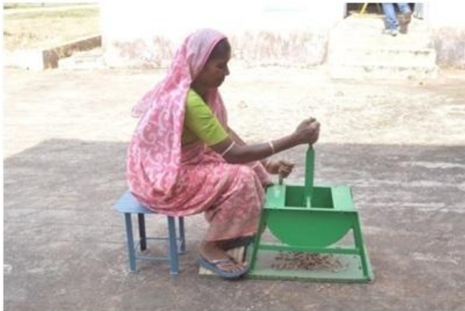
Figure 6: Manually operated groundnut decorticator
