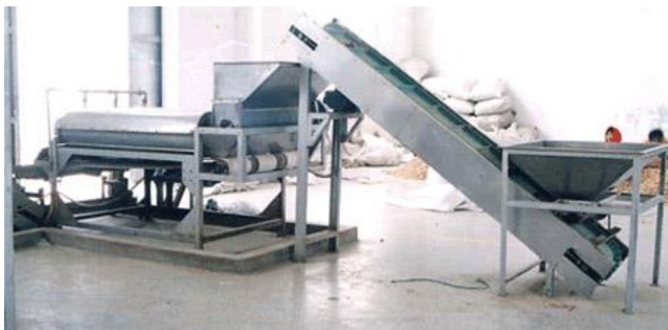
Figure 7: Peanut Cleaning Machine Combined With Elevator Capacity at 800-1500 kg/h
