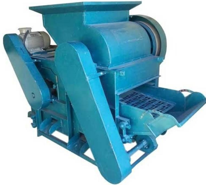
Figure 5: Mechanical groundnut decorticator
