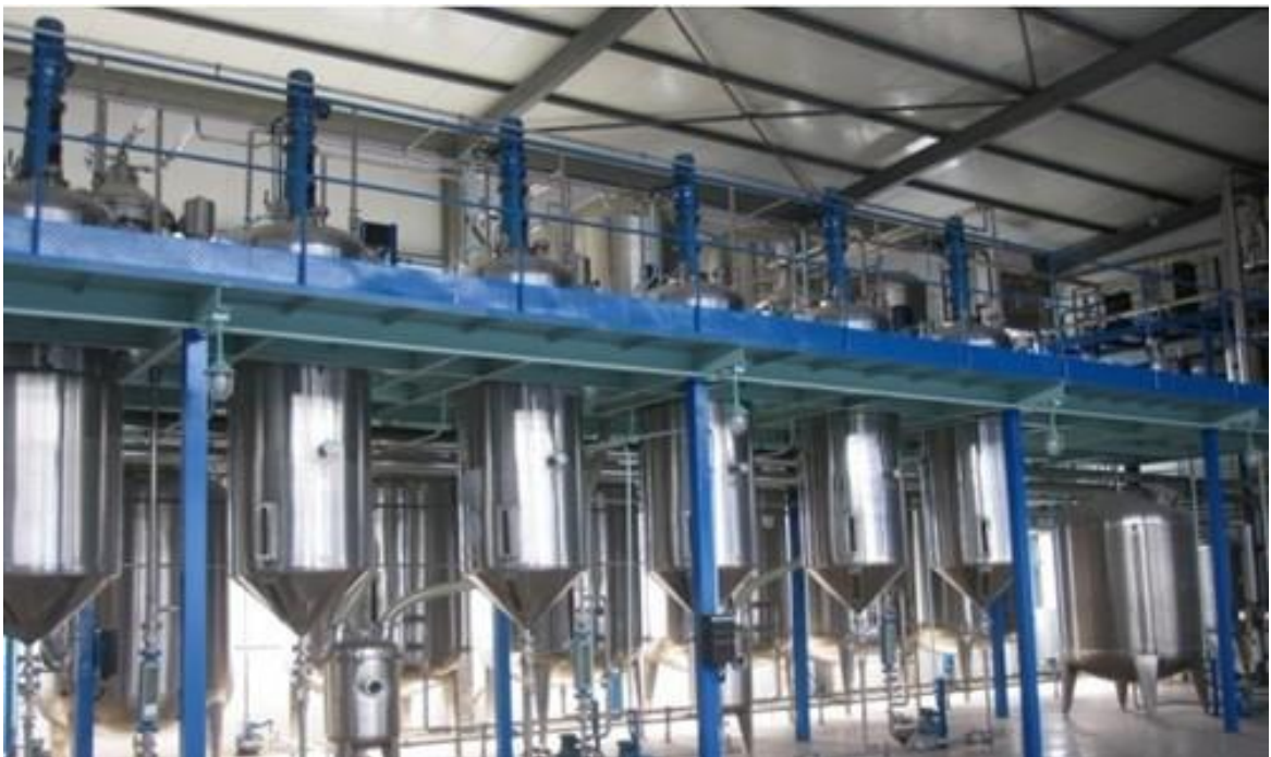
Capsicum Red Pigment Extraction Machinery (5 tons/day)
