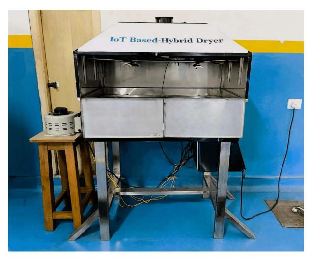
Dryer Capacity: 2.2 kg per batch with 5 mm thickness spreading of papaya pulp
